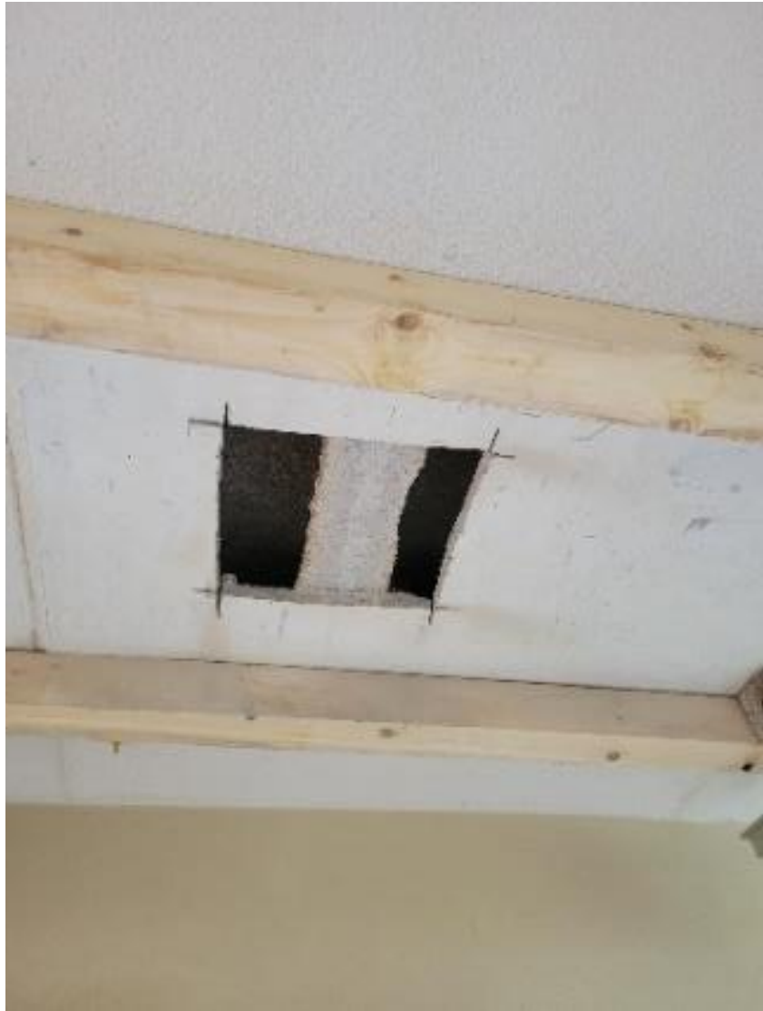
Example of failed test - panel failed clean separation occurred between underside of web and bottom of panel.
