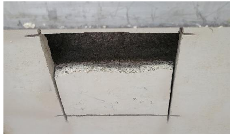
Examples of passing tests – underside of panel stays attached at “web”
